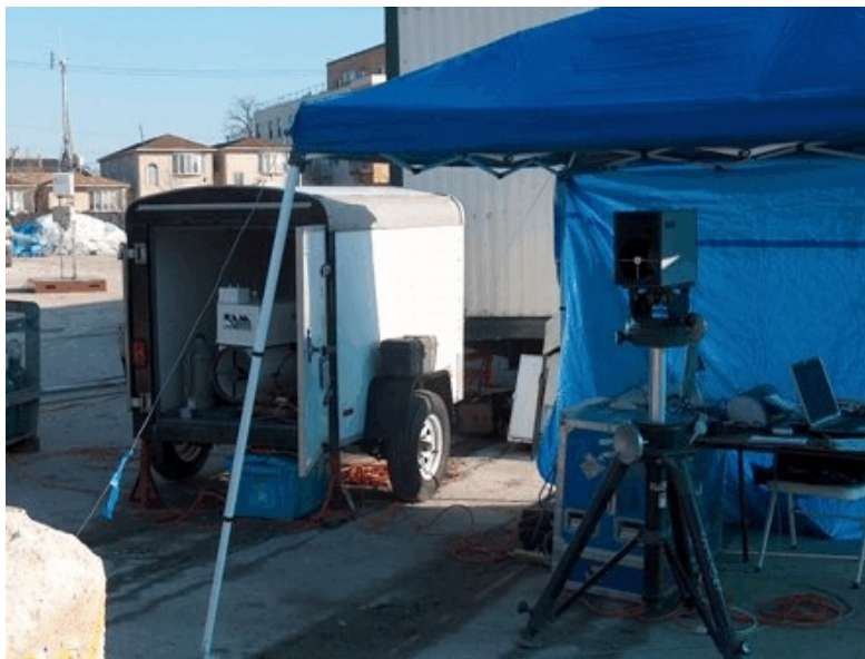
Figure 3. EDO FTIR and IMACC UV Spectrometers at First MGP Site Cleanup
